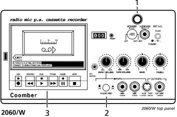
The 2060/W model incorporates a solenoid controlled electronic tape deck and an internal receiver for use with a handheld, lapel or headband type wireless microphones operating on a fixed frequency. In all other respects operation of this equipment is exactly the same as on the 2060 model.
