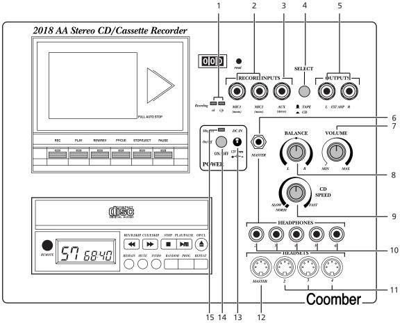
PLEASE NOTE: ALWAYS CLOSE THE CD TRAY WITH THE UNIT SWITCHED ON. PUSHING THE TRAY **CLOSED WITH THE POWER OFF MAY LEAD TO** DAMAGE DURING SUBSEQUENT TRANSPORTATION.
